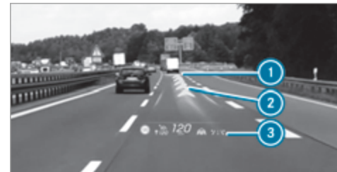
Head-up display with augmented reality (example)
