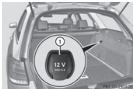
Power socket in the cargo compartment (Wagon)
