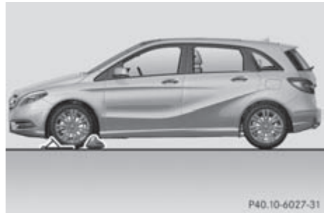
Securing the vehicle on level ground
