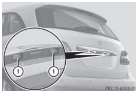
Licence plate lamp (vehicles with halogen headlamps)
