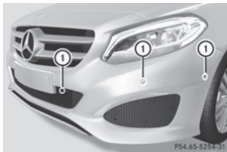
① Example: sensors in the front bumper, left-hand side
