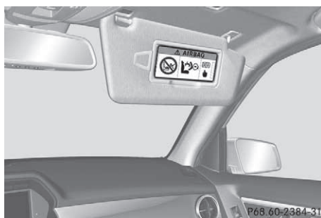
Example: warning notice on the front-passenger sun visor
