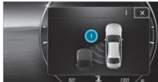
If a course-correcting brake application occurs, the red warning lamp flashes in the outside mirror and a warning tone sounds. In addition, a display
