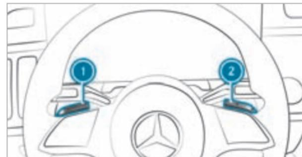
When the automatic transmission is shifted to position **D**, you can manually shift it with the
