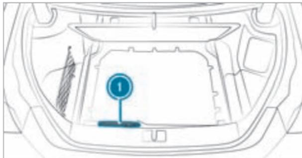
Towing eye ① is located under the boot floor.
