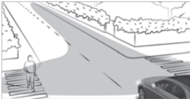
The cornering light improves the illumination of the carriageway over a wide angle in the turning direction, enabling better visibility on tight bends, for example. The cornering light will be activated only when low beam is switched on.
