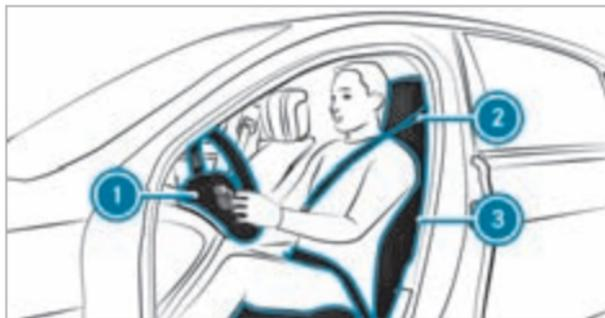
Ensure the following when adjusting steering wheel ①, seat belt ② and driver's seat ③:
