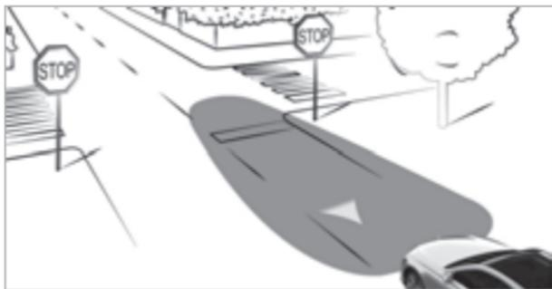
If Traffic Sign Assist detects a corresponding situation, a triangle will be projected onto the road in the following cases at speeds of at least 30 km/h:
