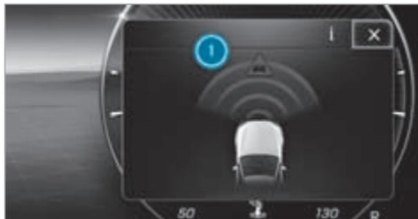
If autonomous braking or situation-dependent brake force boosting has occurred, pop up ①
