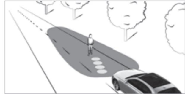
The spotlight function runs in the background and flashes the headlamps in four short bursts at persons detected within the lane markings. You will be made aware of the position of oncoming pedestrians by a projected symbol.
