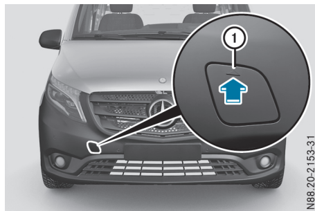
Fixture for the front towing eye in the bumper
