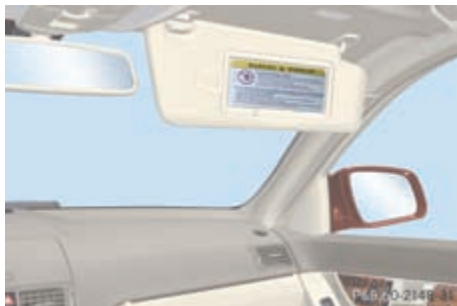
Warning sticker on the front-passenger sun visor
