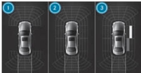
Parking Assist PARKTRONIC display: vehicles without a 360° Camera
