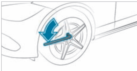
Position of the jack support points
