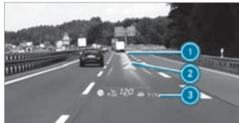
Head-up display with augmented reality (example)
