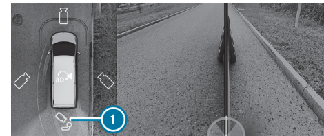
Side view of outside mirror cameras in the trailer view (example)
