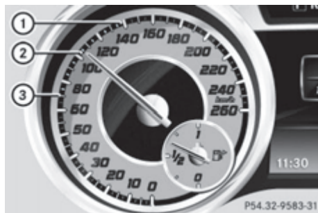
Displaying DISTRONIC PLUS in the speedometer
