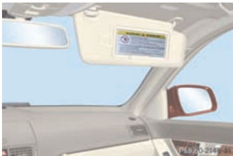
Warning sticker on the front-passenger sun visor
