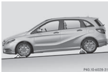
Securing the vehicle on slight downhill gradients
