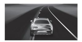
If the front wheel of the vehicle drives over a detected lane marking, this will be highlighted red in the Assistance menu in the driver's display.
