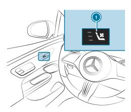
Seat ventilation in the door operating unit in the cockpit (example)
