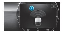
If autonomous braking or situation-dependent brake force boosting has occurred, pop up 1 appears in the driver's display and then automatically goes out after a short time.
