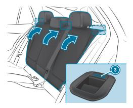
Push seat backrest 2 back to bracket 1 until the backrest engages. If the seat backrest is not engaged and locked in place, red lock verification indicator (3) will be visible.
