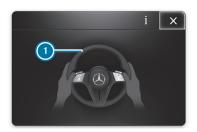
If the system detects that the driver has not steered the vehicle for a considerable time or removed their hands from the steering wheel, an optical warning is given first. Display 1 appears in the driver's display. If the driver still does not steer the vehicle or gives no confirmation to the system, a warning tone sounds in addition to the visual warning message.
