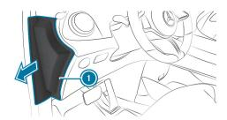
The fuse box is on the driver's side on the side of the cockpit under a cover.
