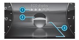
The ECO display shows an evaluation of your driving style on the driver's display depending on the situation. This enables you to check the efficiency of your driving style and adjust it if necessary. The ECO display menu shows a ball that will roll forwards or backwards on a stylised road in the direction of travel according to the driving characteristics.
