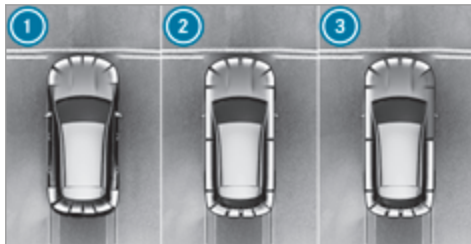
Parking Assist PARKTRONIC display: vehicles with a 360° Camera
