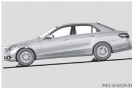
Securing the vehicle on slight downhill gradients
